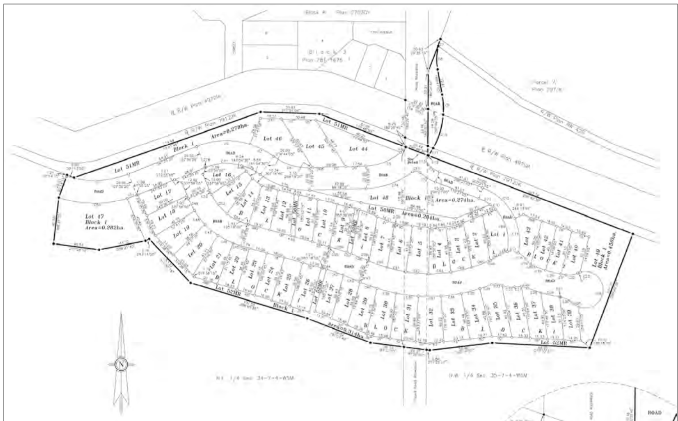
Figure 8 Plan of Survey 0812254 (Southmore Phase 1)
