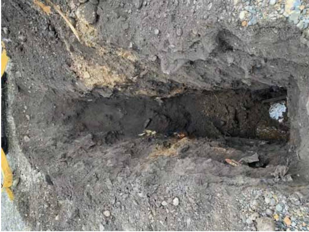
Photograph 48 – Hillcrest Ball Diamond Road – 22HC05, ash, rust-coloured water – 2.9 mbgs. September 22, 2022.
