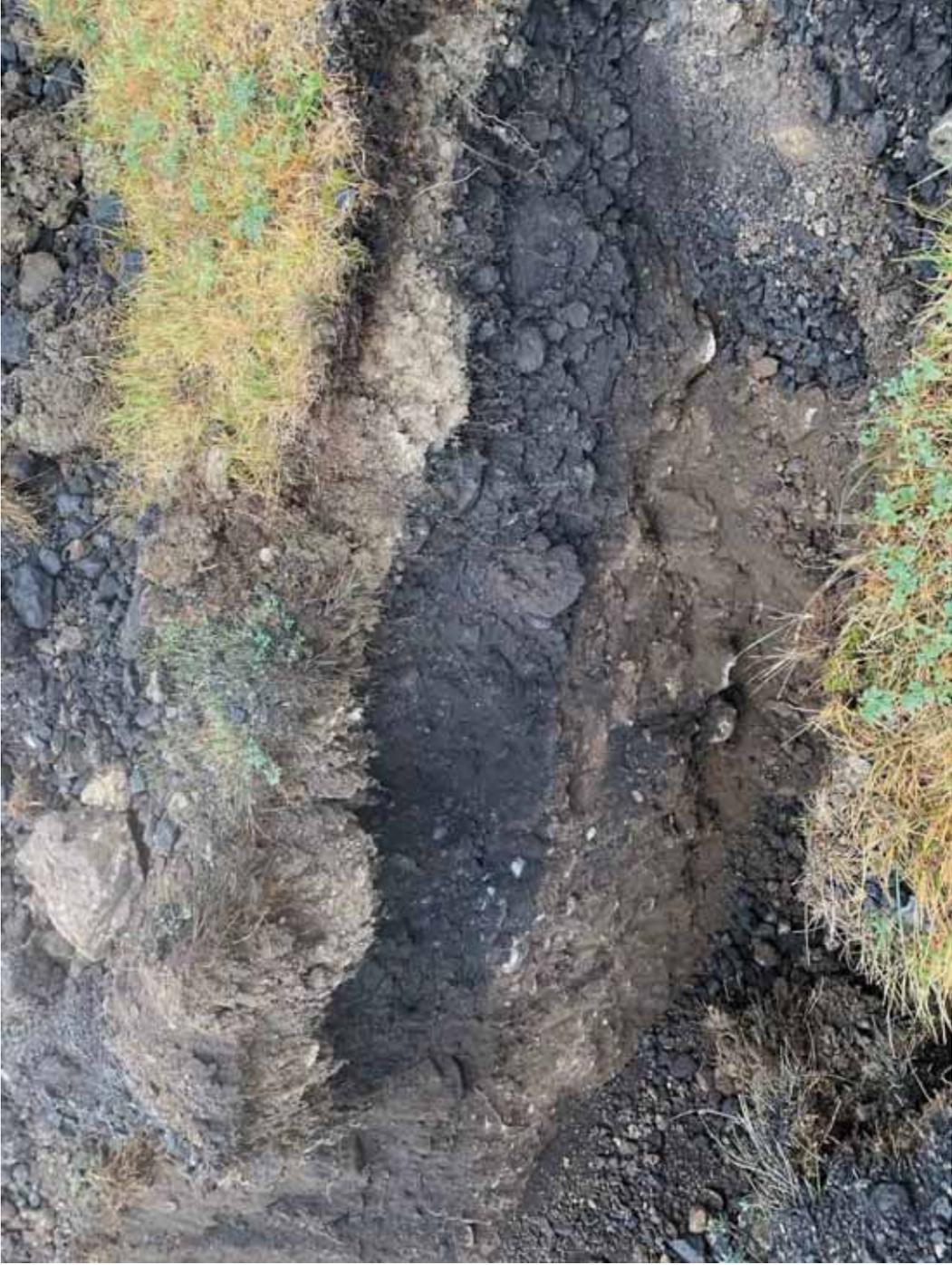
Photograph 45 – Hillcrest Ball Diamond Road – 22HC03, low-grade coal disposal in upper part of test pit.
